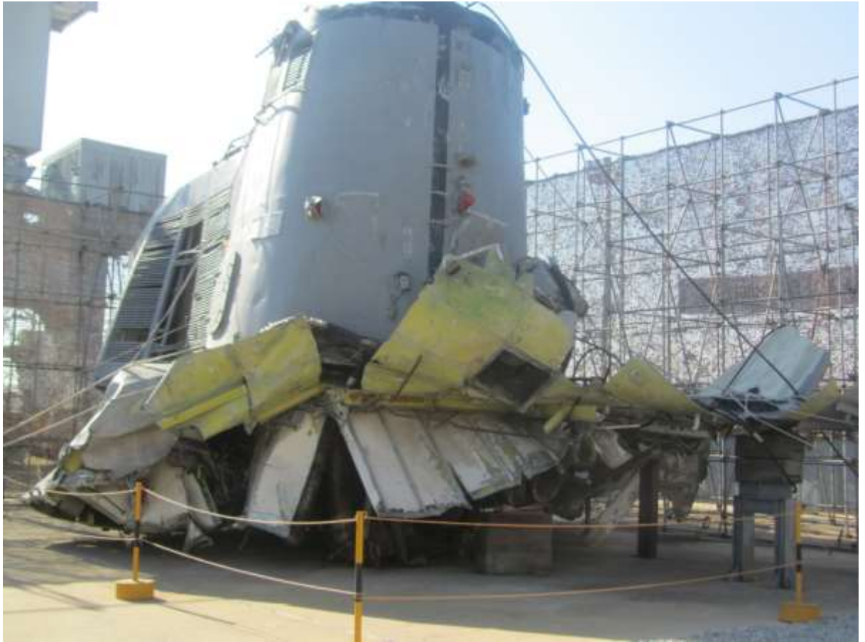
Figure 5-2 – Recovered upper structure wreckage of the sunken Republic of Korea Navy ship Cheonan (photo courtesy of author).
